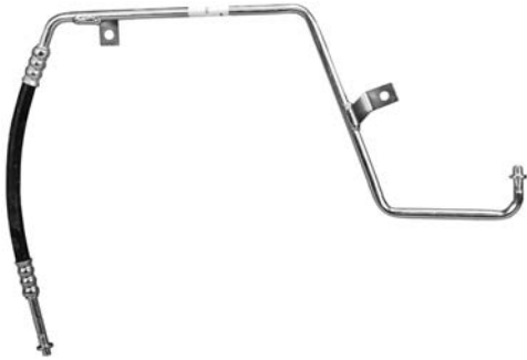
09-0657 LIQUID HOSE / DRIER to CONDENSER Freightliner M2 OE# A22-57504-001
